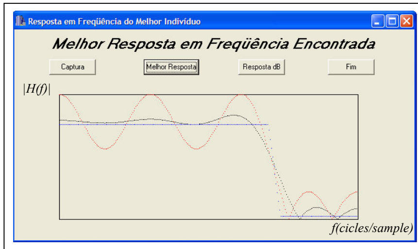
Figure 4: Low Pass Filter, ideal in blue, GA in black, and Parks-McClellan in red.
