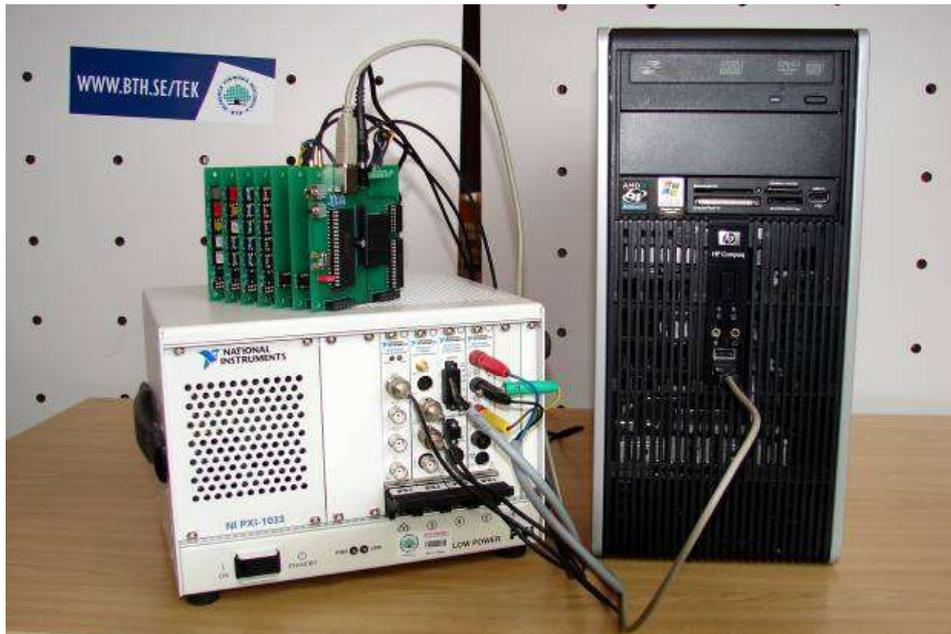
The PXI chassis is NI PXI-1033. The instruments are from left to right function generator NI PXI-5402, dual channel oscilloscope NI PXI-5112, DC power supply NI PXI-4110 with APS-4100, and DMM NI PXI-4070. This equipment is manufactured by National Instruments.
